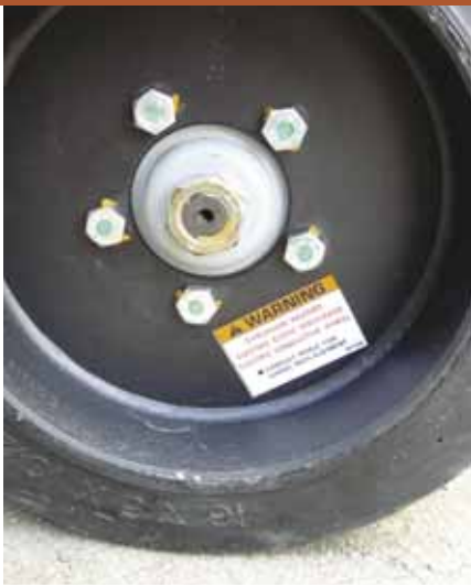
Tires use specially compounded electrically conductive rubber to ground the machine to prevent electric sparks.
