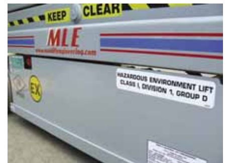
Battery-powered EX scissor lifts typically house the battery box and electric motor inside an explosion-proof box.
